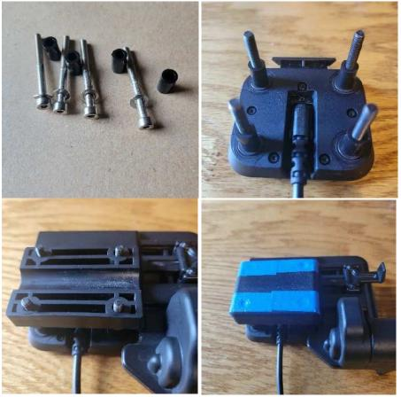
The screws may seem to be a little short, however once they are tightened down and the grommets compress around the mounting bar on the motorcycle you will find the screws are the correct length.
