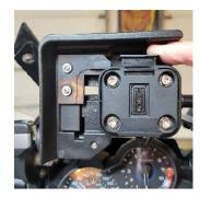
**To remove** the Zumo XT2 from the NAV base, unlock the NAV base and slide the tab all the way to the left. Place your finger into the top right-hand side of the NAV base and push down on the release tab and the Zumo XT2 will now be unlocked and easily removed.
