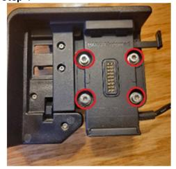
Use a T20 wrench to remove the 4 screws that hold the BMW NAV mount to the accessory bar. The mount will come apart into three pieces: The back plate, the locking mount, and the base plate that the NAV V/VI is attached to. You can set aside the old base for the NAV V/VI.
