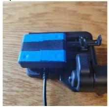
Take four small strips of masking/painter's tape, scotch tape, etc. and place over the four recessed nuts on the backside of the base that holds the BMW mount to the bow or bar that the BMW NAV base is attached to. This will hold the 4 nuts in place throughout the process.
